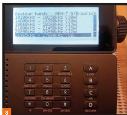
Fig. 8: The fast route to the various bands covered by this radio, including CB.
